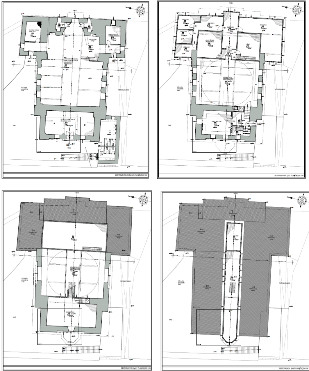
Fig.29-32 - Kemaliye Museum Restoration Project, Ground Floor, First Floor, Second Floor, Third Floor Plans,
